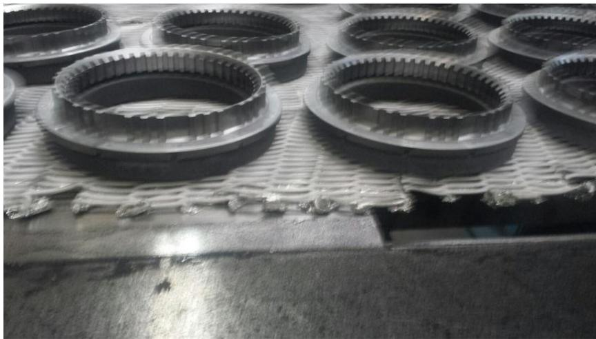
**Figure 1. T314 Stainless Steel Woven Wire Belt with Frayed Edges**
